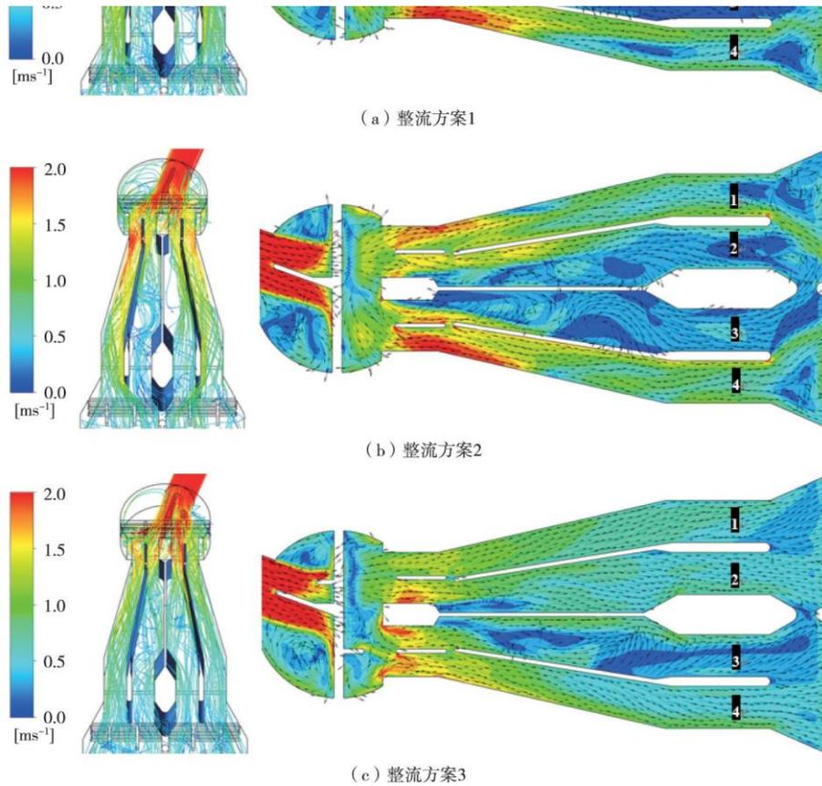
Figure 10 Inlet Flow State of Each Rectification Scheme
