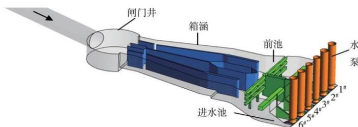
Figure 2 3D Geometric Model of Intake System of Urban Rainwater Pump Station
