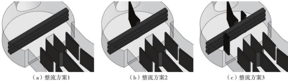
Figure 9 3D Geometric Model of Three Rectification Measures in Gate Shaft of Pumping Station
