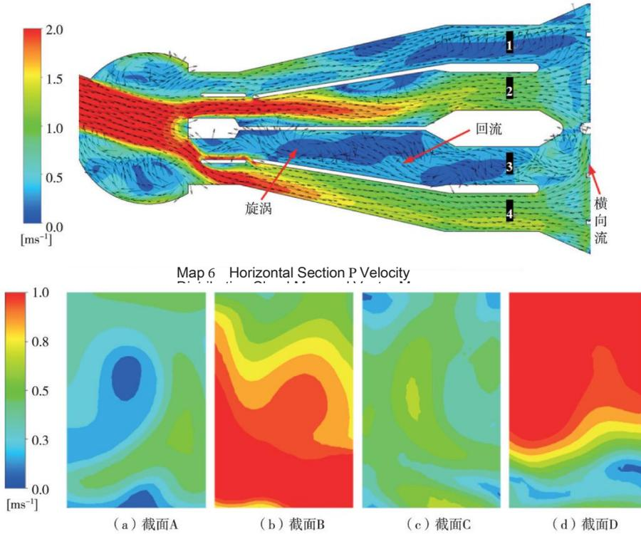
Figure 7 Box Culvert 4 Velocity Distribution Cloud Map of Hole Exit Section
