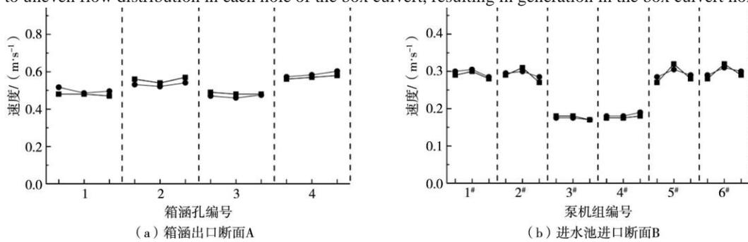
Figure 18 Rectification Scheme 3 Comparison of Velocity Points of Each Measuring Vertical Line in Mainstream Direction
