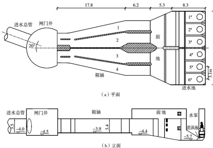
Figure 1 Layout of Plane and Facade of Urban Rainwater Pump Station (Unit: M )
