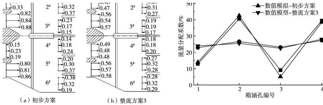
Figure 16 Vertical Average Velocity Distribution of Typical Section Survey Points (Unit: M/S ) Figure 17 Comparison of Flow Distribution Coefficient of Box Culvert Holes
