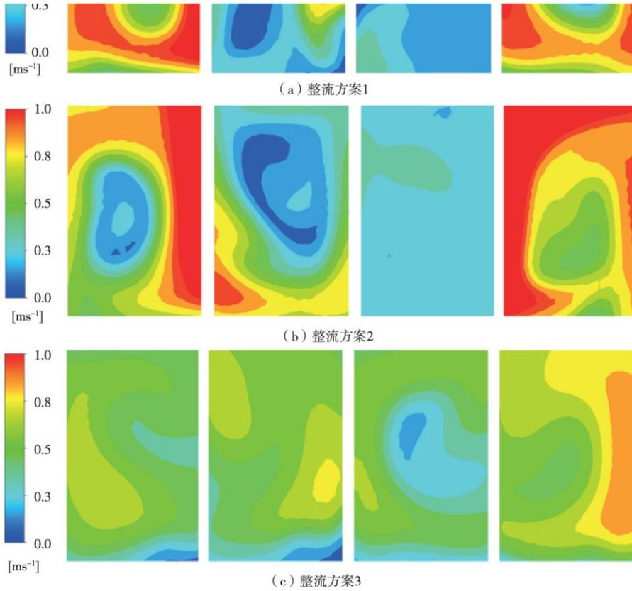
Figure 11 Box Culvert of Each Rectification Scheme 4 Velocity Distribution Cloud Map of Hole Exit Section
