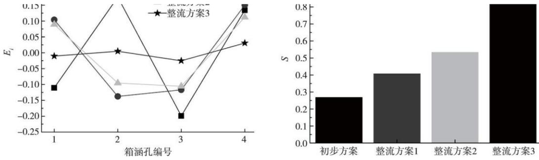
Diagram 12 Flow Distribution Unbalance Value Diagram of Each Hole in Box Culvert 13 Comparison of Total Flow Distribution Uniformity of Each Scheme
