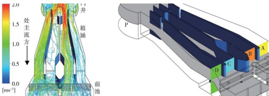
Figure 4 Three-dimensional Streamline Diagram of Preliminary Plan 5 Selected Typical Sections
