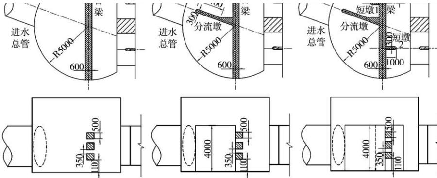
Structural Arrangement of Figure 8 3 Rectification Schemes Designed in Gate Shaft (Unit: mm )
