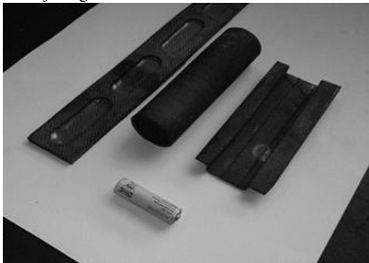
Figure 1. Article samples made of Si-SiC composites (from left
