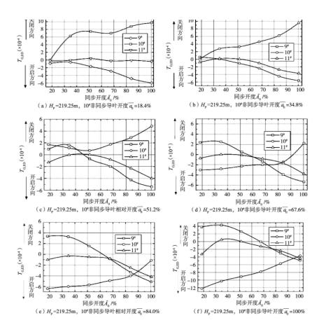
Fig. 5 water moment of asynchronous guide vane
