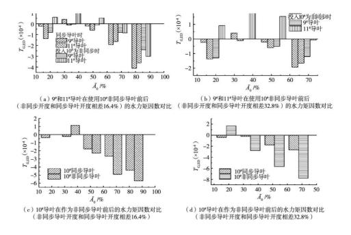
Fig. 6 effect of asynchronous guide vane on water torque of synchronous guide vane
